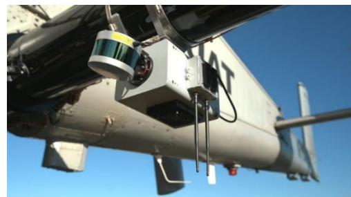
Figure 2: Autonomy System Mounted on the K-MAX. - Courtesy of Near Earth Autonomy
